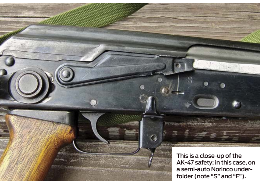
Norinco-made under-folder illustrates many of the classic AK-47 features, including the large lever safety, slanted pistol grip, and mag release in front of the trigger guard.
