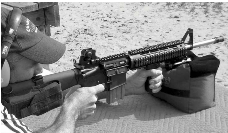
This Rock River A4 Middy HBAR Carbine is fully accessorized and features a free-float quad rail, ladder rail covers, a 1/2 MOA fixed BUIS, stock-mounted spare magazine pouch, Bravo Company M-16 bolt carrier group, Badger Ordnance Tactical Latch, plus a Barska laser and a CAA SVG (short vertical grip) on the lower forward rail section.
